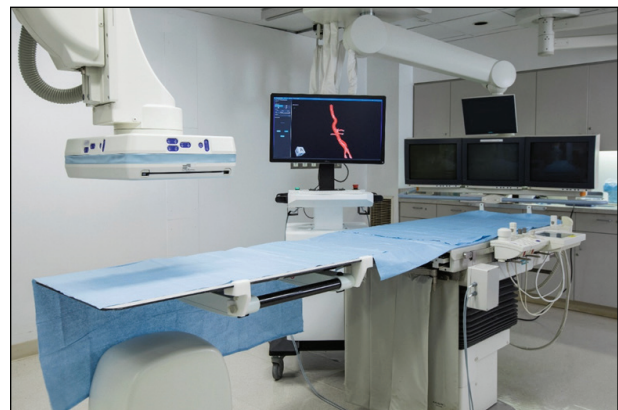
Figure 2. A workstation in a fluoroscopic hybrid operating room. The addition of the workstation is designed to be incorporated into the normal workflow of the endovascular suite, maintaining a relatively small footprint.
