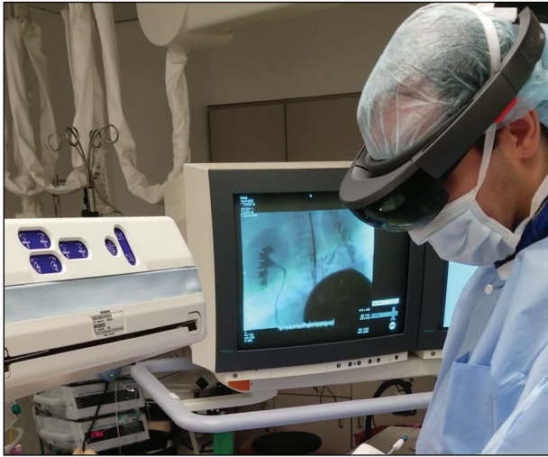
Figure 5. A heads-up display used during EM tracking of a catheter and wire system in a porcine model. This provides a 3D holographic image of the procedure that is taking place.
