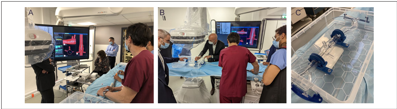
Figure 1. (A) Overview of the setup, with the guidance system integrated to a discovery IGS 730 hybrid room (GE HealthCare, Chicago, IL, USA). (B) A polymer box containing a thoracoabdominal aneurysm model was installed on the imaging table, under which was placed the EM field generator. (C) Because the procedure was almost exclusively performed under electromagnetic navigation, it was not necessary to wear lead for the majority of the experiment. The thoracoabdominal aneurysm model is made from transparent polyurethane.
